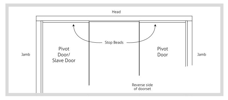
**F.** Once the door stops are fitted, close the doors and mark out positions of the drop bolt keeps on the head, face fix using screws provided (dust box not required). Repeat on any flush bolts for the bottom of the doors.
