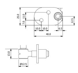
B: Screw in the main body of the bolt into the mounting plate until the back of the hinge flag is approx 1mm from jamb face for optimum adjustment.
