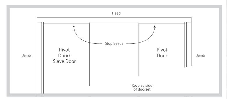
**F.** Once the door stops are fitted, close the doors and mark out positions of the drop bolt keeps on the head, face fix using screws provided (dust box not required). Repeat on any flush bolts for the bottom of the doors.
