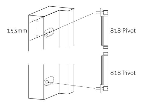
B: Screw in the main body of the bolt into the mounting plate until the back of the hinge flag is approx 1mm from jamb face for optimum adjustment.
