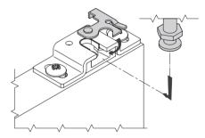
Secure bolt retainer plate.
