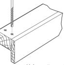
Using a 3mm diameter drill bit, drill 2 holes through the front head and into the jamb to approximate depth of 75mm
