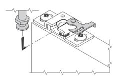
Insert bolt of pivot into plate on leaf.
