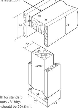
Jamb length for standard imperial doors 78" high (1981mm) should be 2048mm.
