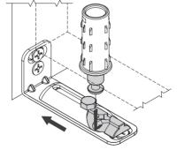
Compress spring loaded pivot & insert into wall bracket. Slide plastic into wall bracket.
