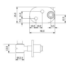
B: Screw in the main body of the bolt into the mounting plate until the back of the hinge flag is approx 1mm from jamb face for optimum adjustment.
