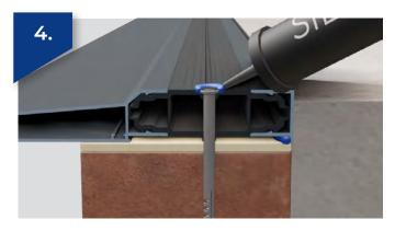
Once you have positioned the cill and made sure it's level, drill & fit through the centre of the thermal break as shown above, using suitable fixings, at the positions shown in point 5 below. Applying a small amount of silicone to fixings to prevent water ingress.
