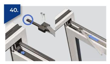
Slide & click the guide into position at the hinge end of the sash head.
