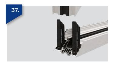
Mitred corners are constructed using 2 corner cleats that fit into locating channels in the aluminium profiles. First fit the cleats into one length of profile using a T25 Torx driver. The Torx driver fits through the pre-drilled holes as shown right. Tightening the fitting will draw the corner cleat into place. Fit the next length to form a corner using the same method.
