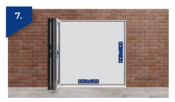
Position frame (along with any optional integral cill or low threshold) into the opening ensuring it's square and plumb, and pack accordingly using frame packers. Also check diagonals are within +/- 1mm. Open doors and support the sashes. Alternatively sashes can be removed as shown on page 11.
