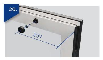
These magnet positions below are for doors with single rollers. Fix 207mm in from edge of the sash. For vertical positioning please see point 22 below.
