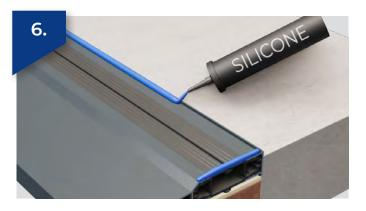
Once the cill is fitted apply a bead of silicone sealant at each end of the cill and along the inner edge of the upstand.
