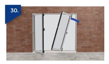
For track bound doors release the espag handle and slide the doors towards the hinged jamb until the central hinges are exposed. Remove the screws and remove the sash by supporting at the hinged jamb and sliding away from the hinged sash. This can then be removed by angling the sash until the top guide disengages from the track. Carefully lift the sash out of the bottom track until the roller is clear and place securely out of the way to prevent damage.
