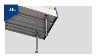
Secure the frame to the threshold using the supplied 4.8 x 55mm screws through the pre-drilled holes. Secure the top of the outerframe using the same method.
