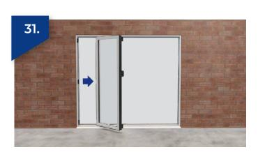
The final sash can be removed from the hinges by removing the three screws in each hinge as before, fully supporting the sash while this is done. Lift carefully and place securely out of the way to prevent damage.
