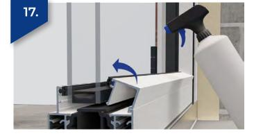
We advise spraying the unit with a mild soap/water mixture or glass cleaner to make beading easier. Ensure you have toe & heeled/packed the unit correctly as shown on page 8. Fit the top bead in place to secure the glazed unit (rotating the beads until they clip in to place as shown above). Next, fit the bottom bead.
